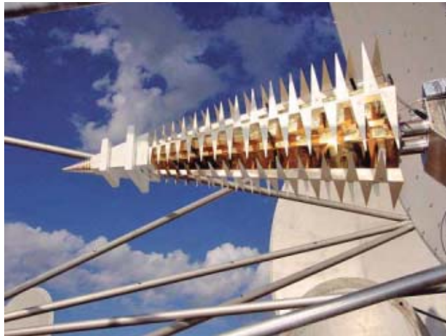
[FIG2] This log periodic dual polarization feed covers 0.5–11.2 GHz. Each of the feeds from the 42 telescopes in the array outputs an equivalent of 200 GB/s.
